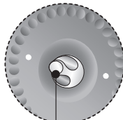
⑤ When you fix the rubber packing into the detachable cover, hold it between and put it in the edge of the detachable cover by turning it.
